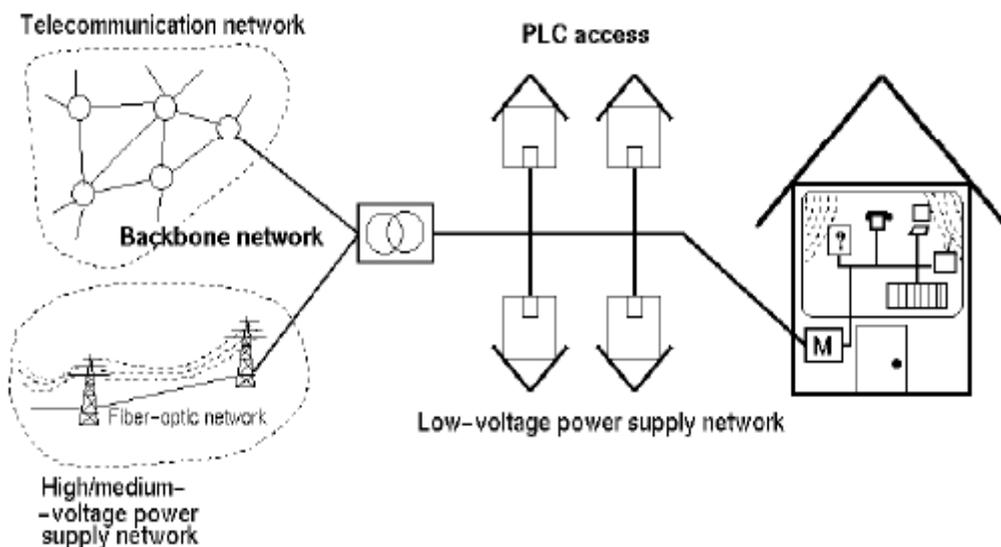
Figure 2.12: PLC Access Network (Source: Hrasnica *et. al.*, 2004)
