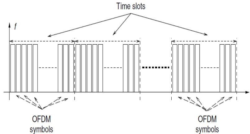
Figure 2.6: OFDMA/TDMA (Source; Hrasnica *et. al.*, 2004)
