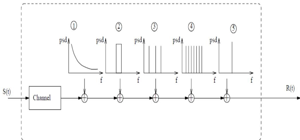
Figure 2.15: The additive noise in the Powerline Environment (Source: Hrasnica *et. al.*, 2000)
