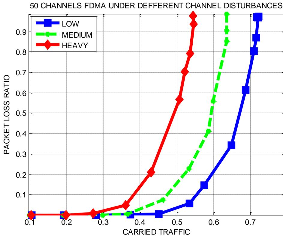
Figure 4.1: 50 Channels FDMA under different conditions
