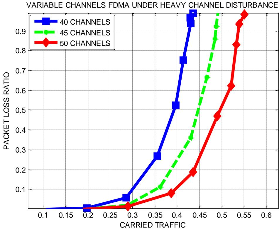
Figure 4.2: Variable Channels under Heavy Channel Disturbance
