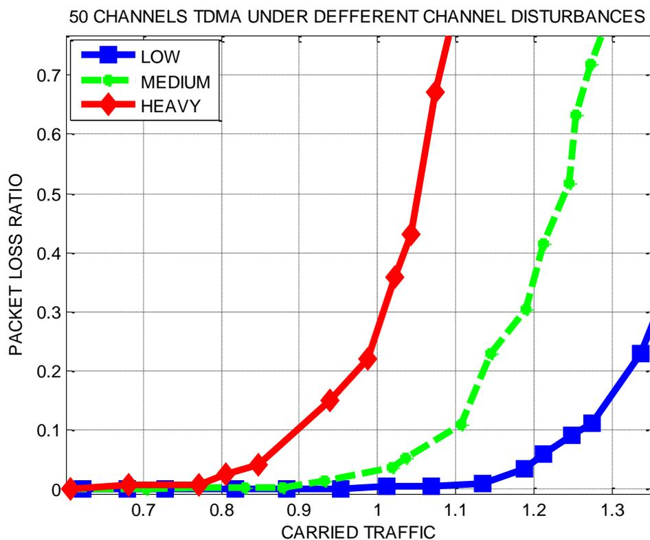
Figure 4.3: 50 channels TDMA under different channel disturbances
