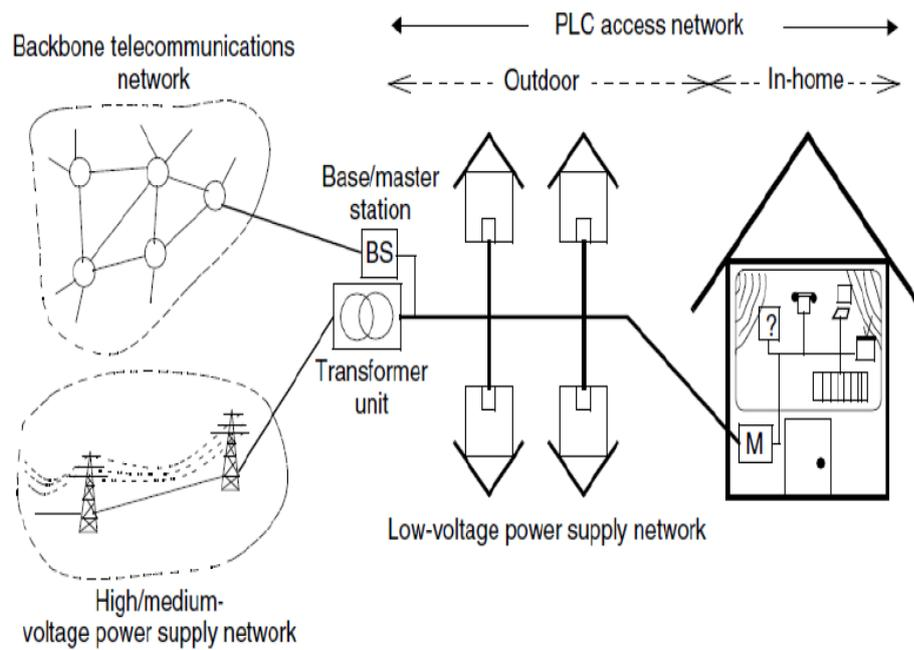
Figure 2.1: Structure of PLC (Source: Hrasnica *et. al.*, 2000)
