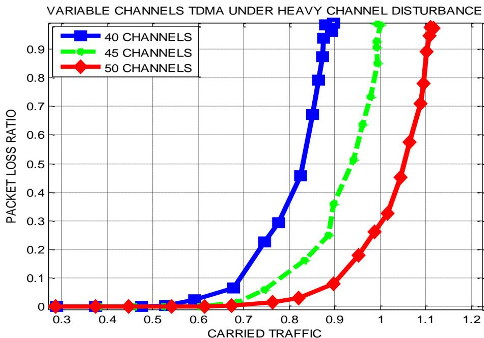
Figure 4.4: Variable channels TDMA under heavy channel disturbances
