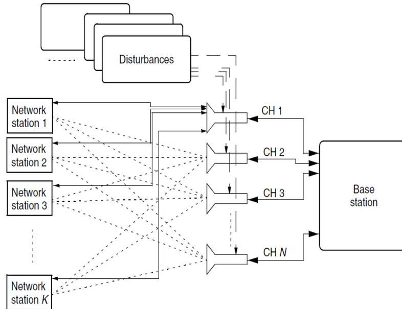
Figure 2.18: PLC Simulation Model (Source: Hrasnica *et. al.*, 2000)
