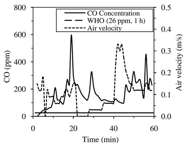
Fig. 6 Effect of air velocity on CO concentration during cooking.
