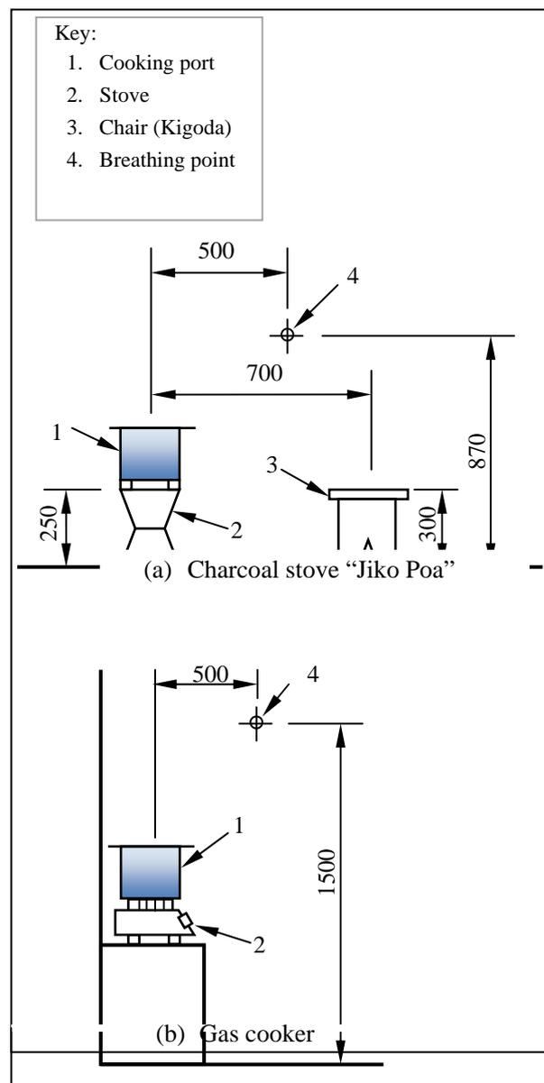
Fig. 1 Schematic diagram of the experimental layout using (a) charcoal stove “Jiko Poa”; (b) gas cooker.
