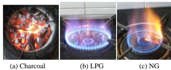
Fig. 4 Flame structures of different types of fuels.
