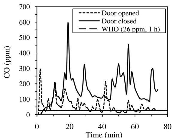
Fig. 5 The effect of closing the kitchen door on CO concentration.
