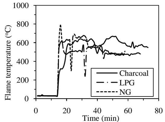
Fig. 3 Flame temperature profile of different types of fuels.
