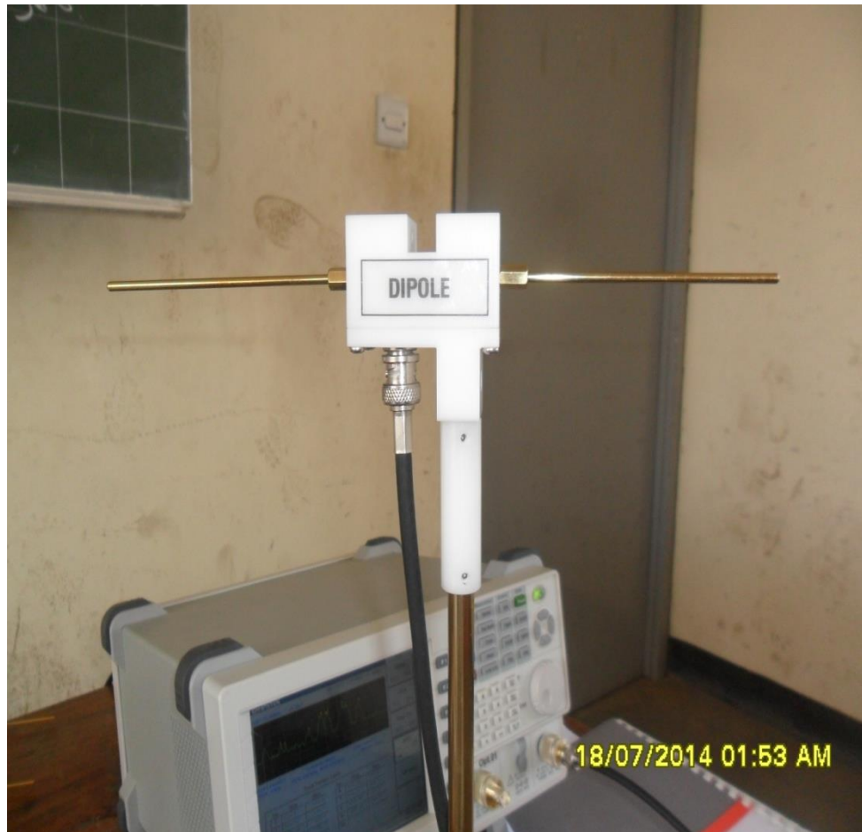
Figure 3: Open Dipole Antenna
